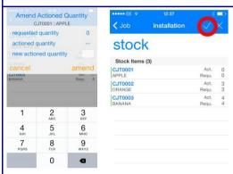
5. An installation task is the 1st task here, tap on each stock item, enter the quantity of stock that you have installed, if they do not match required add a comment then tap the tick icon.
